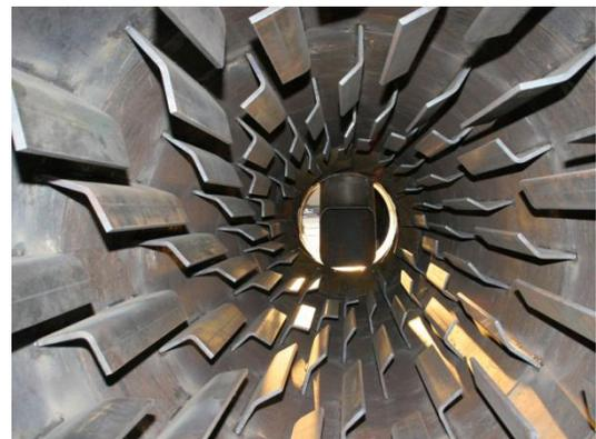
Diagram: The diagram above illustrates how flights create the curtain in a rotary dryer to maximize heat transfer
