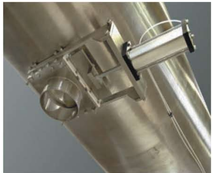
Bottom Discharge Outlet with Pneumatic Operated Slide Gate Valve
