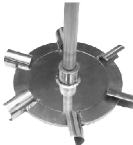
Mostly used for gas dispersion application. Curve blade (Concave, parabolic etc.) disc can handle 2 to 6 times more gas than flat blade disk turbine. Power drop between gassed and un-gassed condition is very less than conventional flat blade disk impellers. Hence it is preferred choice for gas dispersion application viz. Fermentation, Hydrogenation, Oxidation, Carbonisation, Ethylation etc.
