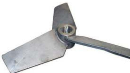
These are most efficient axial flow impeller. It is recommended for blending, solid suspension, heat transfer etc. It provides maximum flow at minimum power. Mostly available in three blade version. But different number & width of bade are also common in special applications. This is also called as fabricated propeller.
