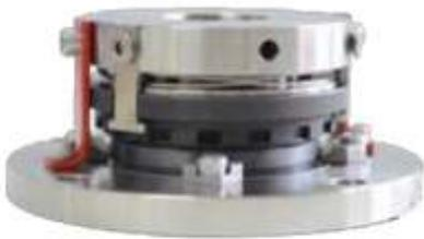
A single mechanical seal consists of two very flat surfaces that are pressed together by a spring and slide against each other. Between these two surfaces is a fluid film generated by the product. This fluid film prevents the mechanical seal from touching the stationary ring. An absence of this fluid film (dry running of the pump) results in frictional heat and ultimate destruction of the mechanical seal.
