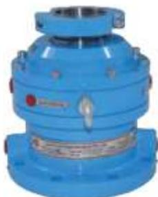
A double mechanical seal consists of two seals arranged in a series. The inboard, or "primary seal" keeps the product contained within the housing. The outboard, or "secondary seal" prevents the flush liquid from leaking into the atmosphere.
