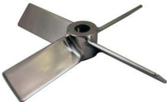
These are axial mixing impeller with considerable amount of radial flow. It produces suction when placed near the liquid surface. Hence used for blending of immiscible liquids, solid incorporation etc. It is also a preferred choice for applications where the viscosity change during the process is large. These are mostly available in four blades @ 45 degree. But different numbers of blade with various angles are also used depending on application.
