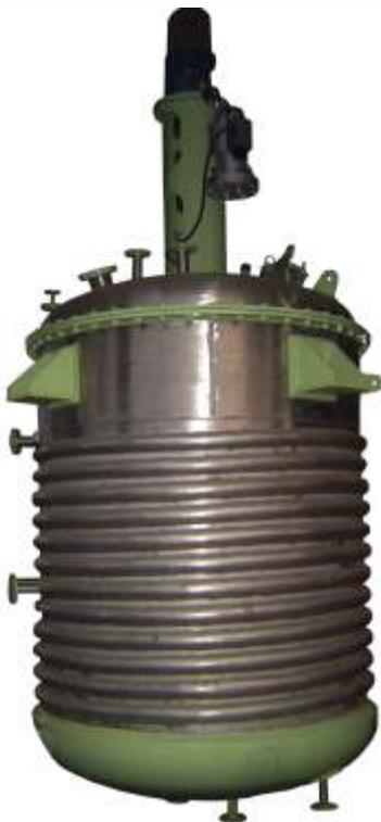
Standard Reaction vessels are designed for 3-4 kg/Cm<sup>2</sup> internal pressure or full vacuum. Reaction Vessels with Jackets are designed for pressure inside the jacket at 3-4 kg/Cm<sup>2</sup>. Reaction vessels for higher operating pressures are also available as per process requirement.
