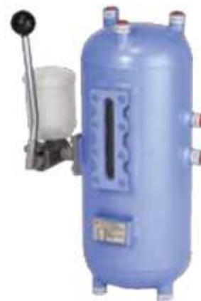
Thermosyphon Vessel is used as a storage & unpressurising unit. Used for double mechanical seals in tandem seal arrangement. This is equipped with cooling coil inside the shell to bring down the temperature of buffer fluid coming from seal to Thermosyphon Vessel.
