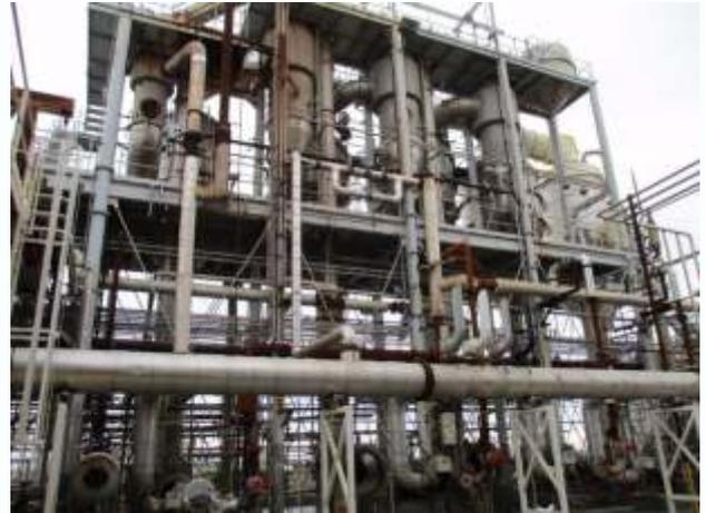
If we consider the heat balance of a single-effect evaporator we find that the heat content (enthalpy) of the evaporated vapour is approximately equal to the heat input on the heating side.
