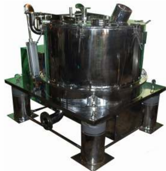
4-Point Mounting with Inertia Plate & Anti Vibration Mounts
