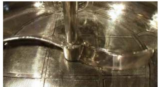
1. **Clock wise rotation:** For smoothing cake surface and compacting it during filtration.
