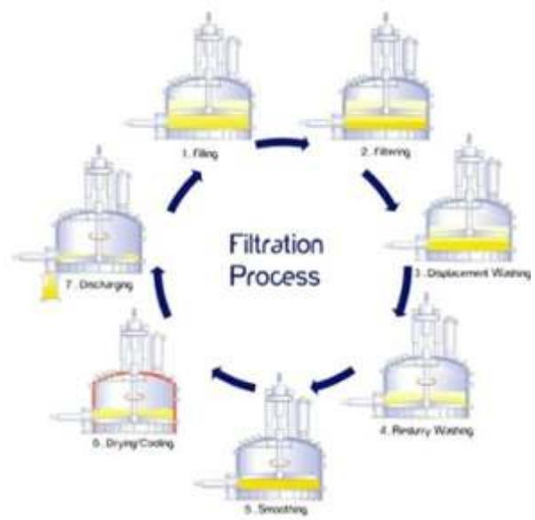
Filtration and drying are critical operations in a variety of industrial processes that require the separation of solid matter from a liquid. Solids can be discharged directly into a dryer, or in the case of a filter/dryer, the drying function is performed using the same equipment.
